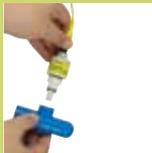
3. Insert the Oxygen Sensor into the Quick-Ox.
